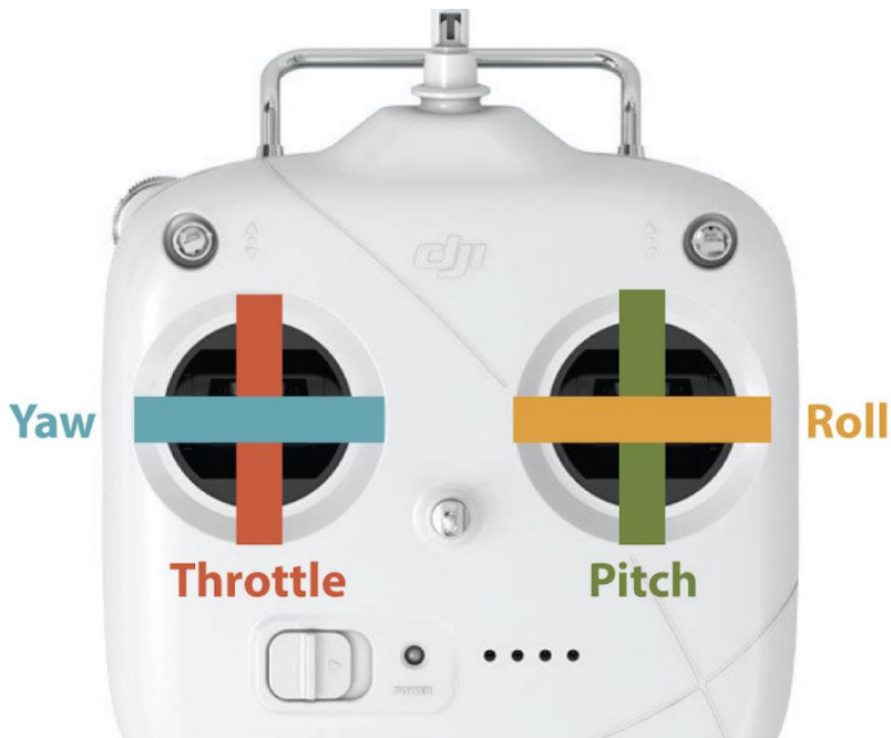
Throttle, Pitch, Roll, and Yaw on a Remote-Control with Two Joysticks. [fromwhereidrone.com]
